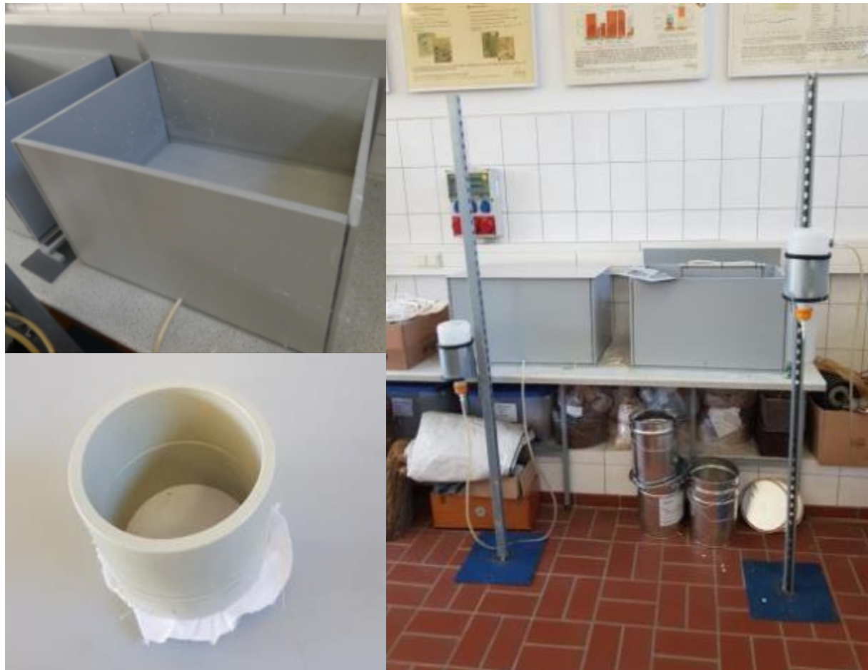
Figure 7. Soil water tension measuring box (top left), sample container (bottom left), complete system including water drainage system (right). [Source ATB]
