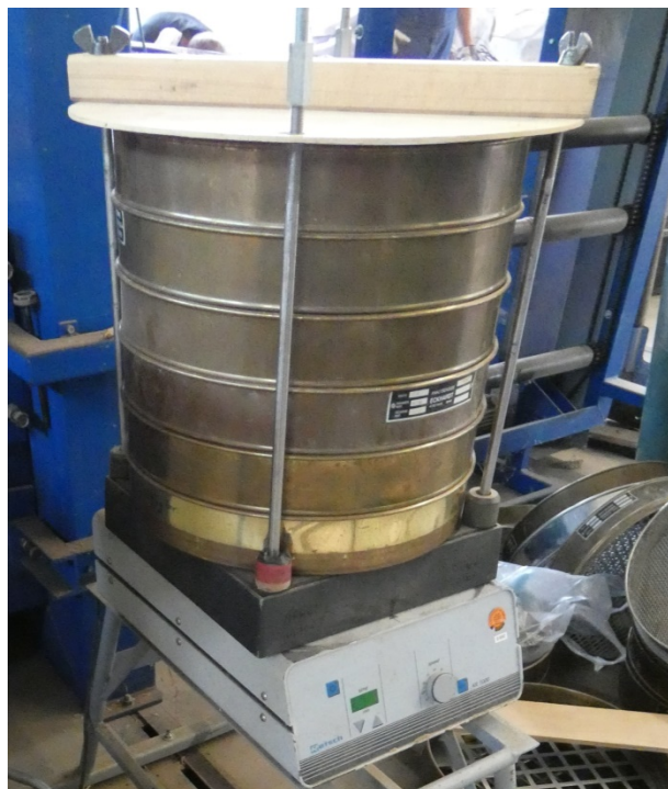
Figure 9. Sieving tower [Source ATB]
