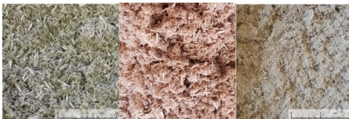
Figure 4. Poplar wood chips after extrusion and blow drying. Left side (coarser end product) extruded at 40 mm aperture opening, middle image (medium coarse product) at 25 mm, right side (finer end product) at 15 mm. [Source: ATB]
